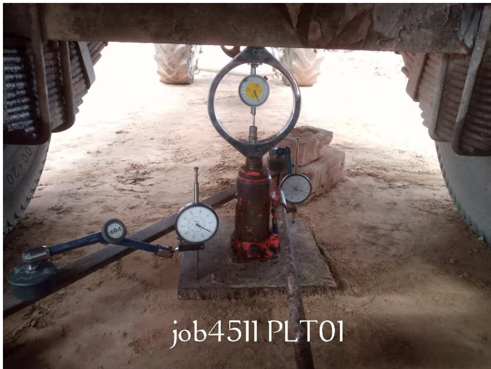
PHOTOGRAPHS SHOWING PLATE LOAD TEST UNDERPROGRESS
